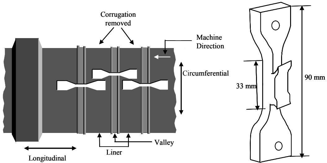
Figure 2 – Location and configuration of pipe junction specimens
