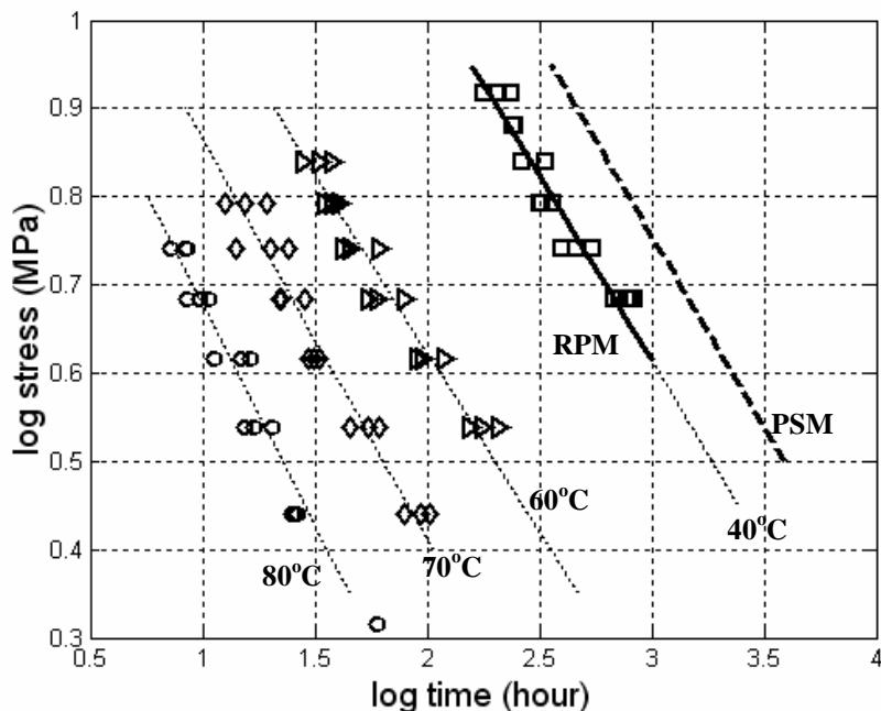
Figure 3 - Experimental and predicted brittle curves on notched pipe liner tests in water
