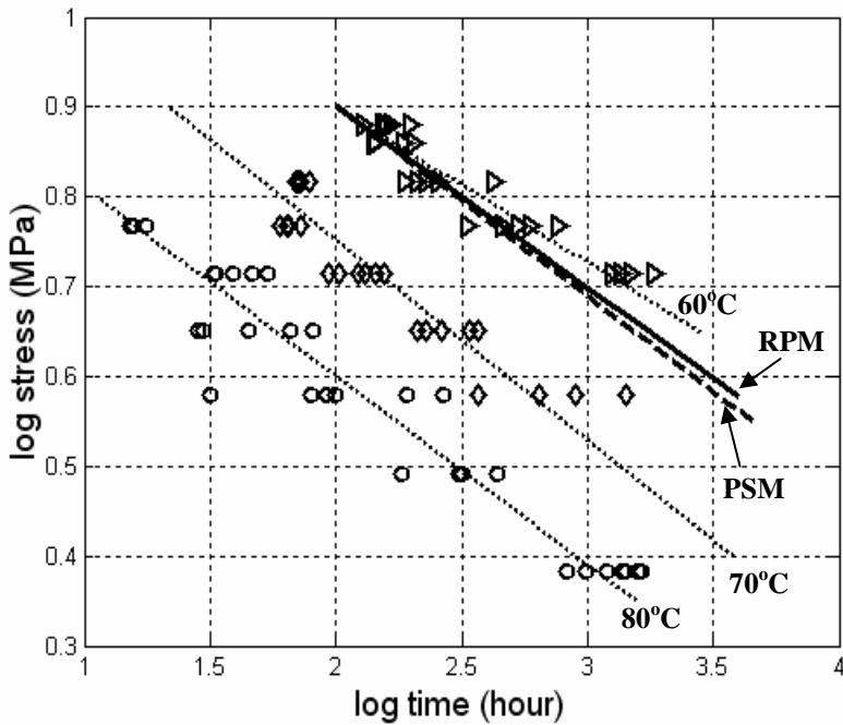
Figure 4 - Experimental and predicted brittle curves on pipe junction tests in water
