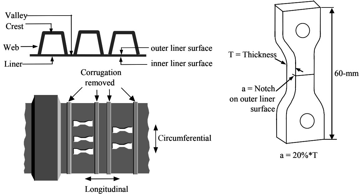
Figure 1 – Location and configuration of the NCLS test specimen on pipe liner
