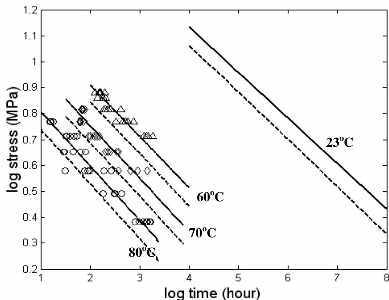
Figure 5 – Predicting the junction brittle curve at 23°C
